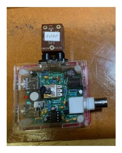
was. I will keep pounding out the CQs until I connect with someone. (www.ReverseBeacon.Net) I did modify this Pixie by taking out the 7.023 crystal and attaching an FT-243 crystal socket Now I can roam the 40-meter CW section with impunity with my collection of 40-meter crystals.
